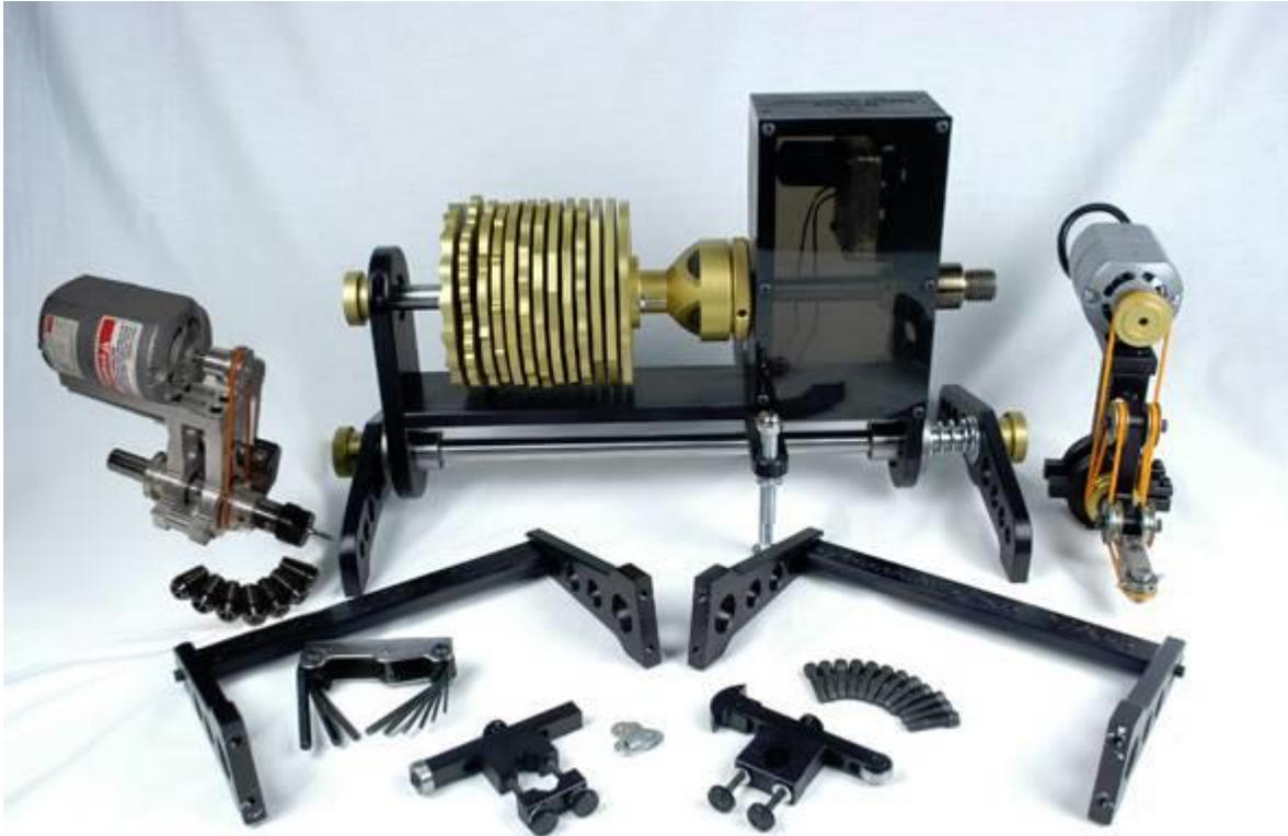
The Mandala Rose Engine is manufactured of 6061 aircraft aluminum and steel.
